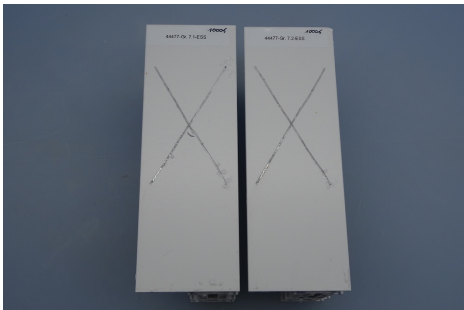
Figure 4 – Group 7 after 1000 h AASS-Test
