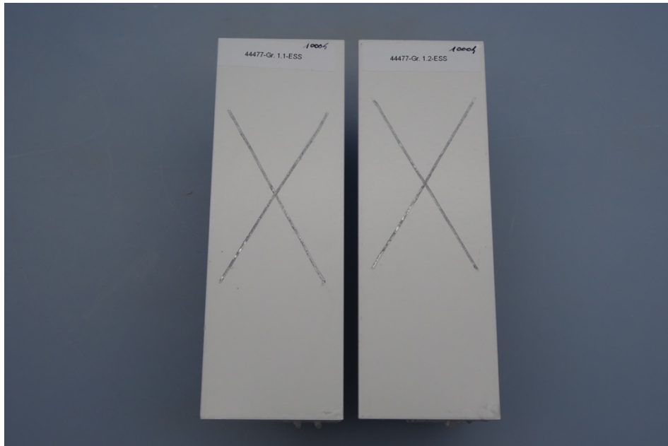
Figure 1 – Group 1 after 1000 h AASS-Test
