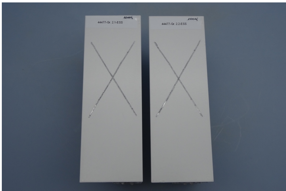
Figure 2 – Group 2 after 1000 h AASS-Test
