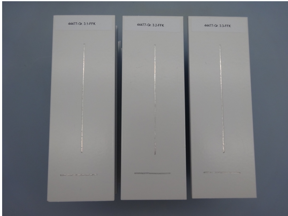
Figure 7 – Group 3 after 1000 h FFC-Test
