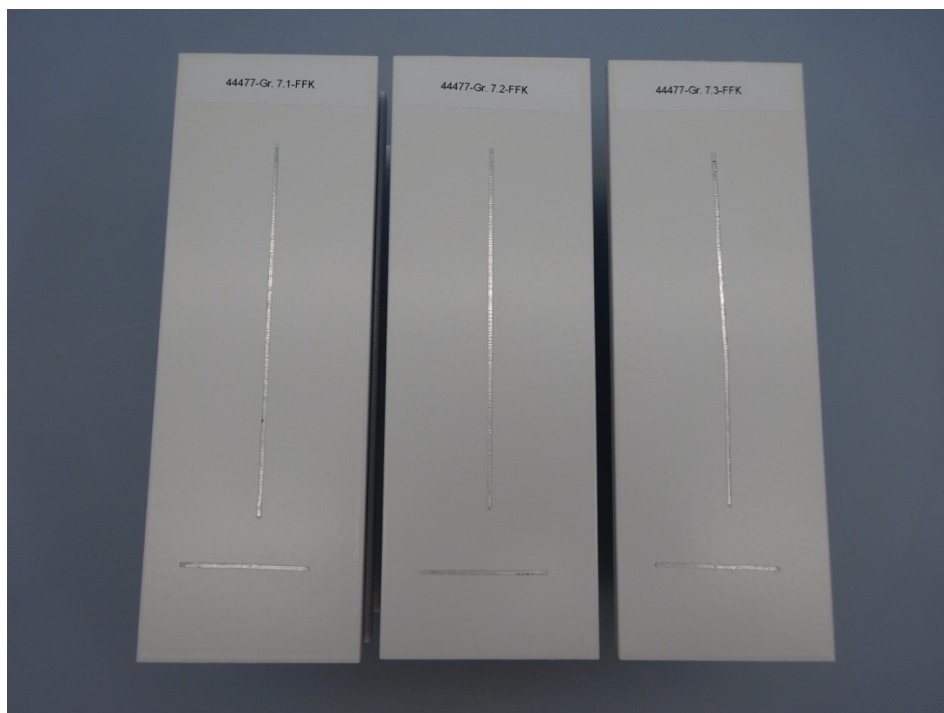
Figure 8 – Group 7 after 1000 h FFC-Test
