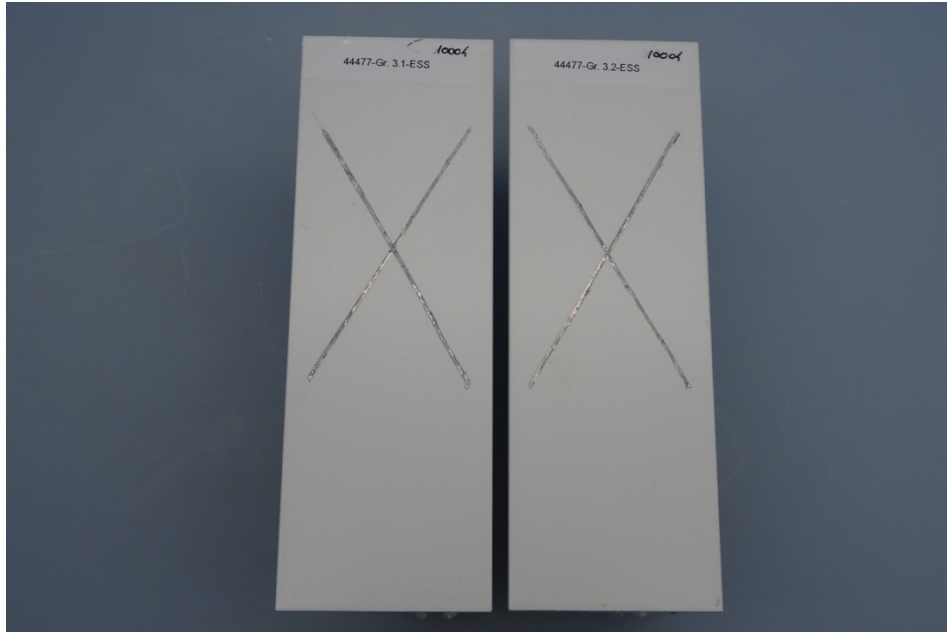
Figure 3 – Group 3 after 1000 h AASS-Test
