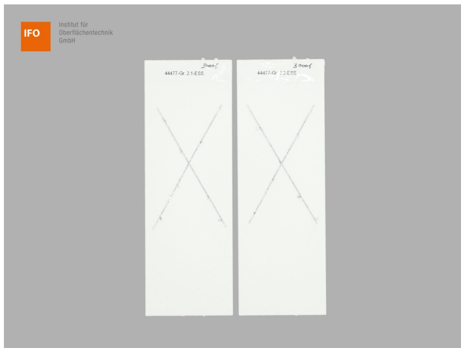
Figure 2 – Group 2 after 3000 h AASS-Test
